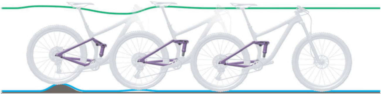
Figure 80: Rear frame damper rebounding too quickly
