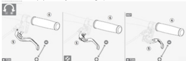
Figure 43: Adjusting the grip distance on a Magura disc brake lever
