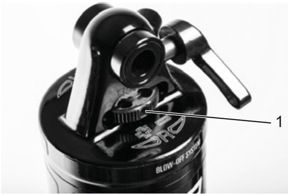
Figure 81: Turning the rebound damper clockwise
