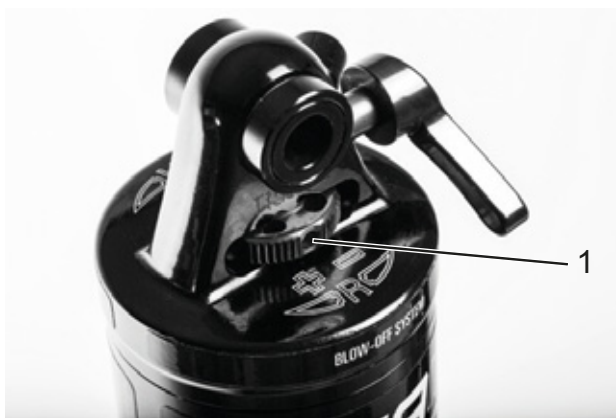
Figure 83: Turning the rebound damper anti-clockwise
