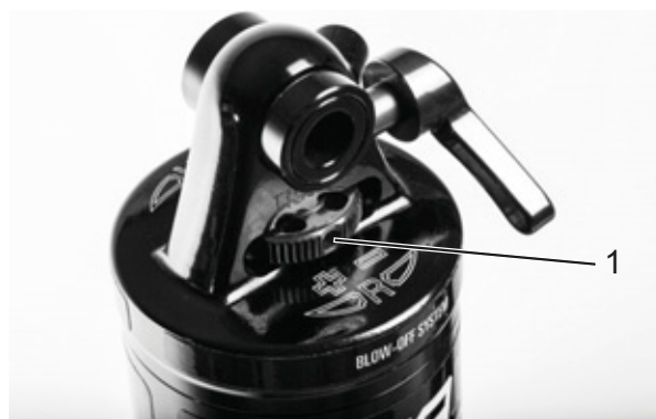
Figure 51: Suntour rebound adjuster wheel (1) on the rear frame damper
