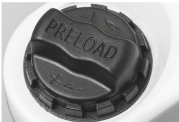
Figure 45: Sag setting wheel on the suspension fork crown
