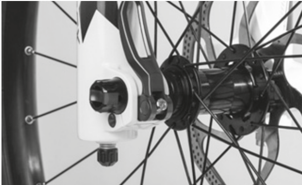
Figure 67: Adjusting the quick release clamping force
