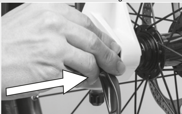
Figure 33: Pushing the quick release in
