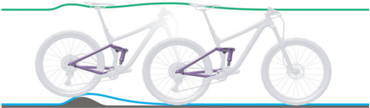
Figure 86: Excessively hard damping in the rear frame damper on bumps
