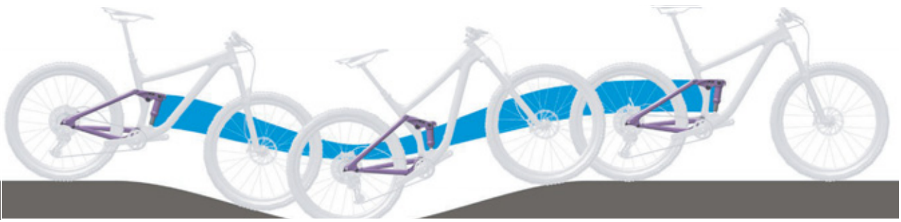
Figure 84: Excessively soft suspension in the rear frame damper on hilly terrain
