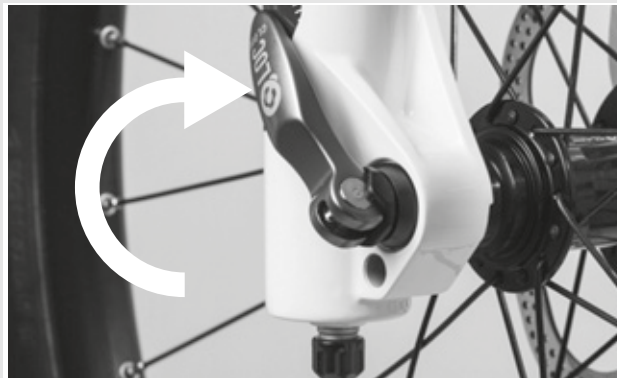
Figure 35: Closing the quick release
