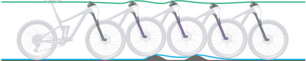
Figure 267: Suspension fork rebounding too slowly
