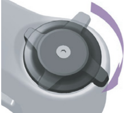
Figure 171: Changing compression adjuster to a harder setting
