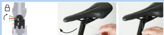
Figure 232: Closing the height adjustment
