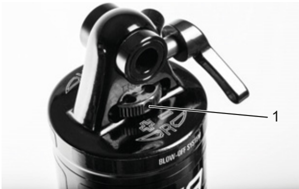
Figure 276: Suntour rebound adjuster wheel (1) on the rear frame damper
