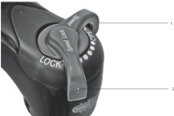
Figure 262: Changing compression adjuster to a harder setting
