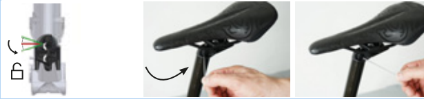
Figure 195: Moving height adjustment to the “Open position”
