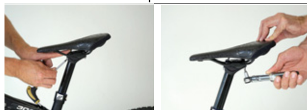
Figure 100: Securing the front and rear screws
