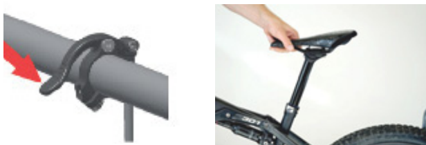
Figure 94: Extending the hydraulic gas pressure spring
